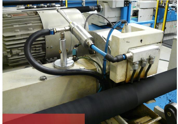
Vortec cooling during grinding of rubber hoses
