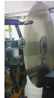
*Vortec cooling of the cutting blade during converting (tissue) paper*
