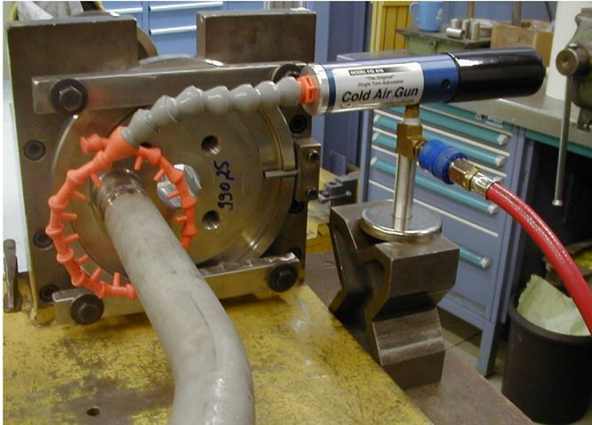
Vortec cooling during/after welding
